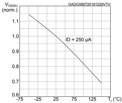
Figure 9. Normalized gate threshold vs temperature
