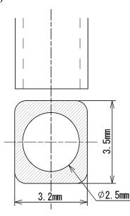
%Nozzle with chamfering is recommended
