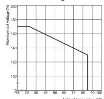
Ambient temperature (°C) Note. The maximum coil voltage refers to the maximum value in a varying range of operating power voltage, not a continuous voltage.
