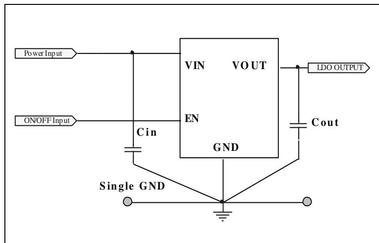
Note:  $C_{in}$  and  $C_{out}$  are  $0.47\mu F$  low ESR ceramic capacitors
