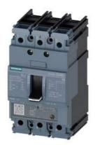
circuit breaker 3VA5 UL frame 125 breaking capacity class S 25kA @ 480 V 3-pole, line protection TM230, FTAM, In=50A overload protection Ir=50A fixed short-circuit protection li=5...10 x In nut keeper kit on both sides
