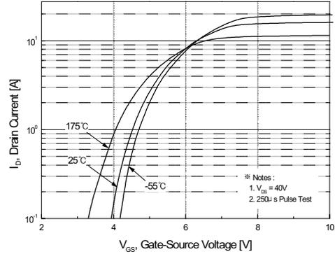
Figure 2. Transfer Characteristics
