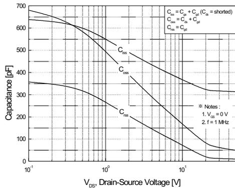
Figure 5. Capacitance Characteristics
