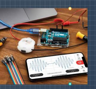
Pokit measures, displays and logs a wide range of parameters including voltage, current, resistance and temperature. It also provides a continuity and diode checker. Pokit is ideal for low voltage electronics, automotive applications, home automation, and more.
