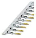
Crimp contact, Pin, rolled, Taped articles, number of pieces per reel: 500, contact diameter: 1 mm, crimp range: 0.08 mm<sup>2</sup> ... 0.22 mm<sup>2</sup>
