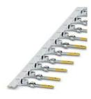
Crimp contact, Pin, rolled, Taped articles, number of pieces per reel: 10000, contact diameter: 1 mm, crimp range: 0.08  $\rm mm^2 \dots 0.22~\rm mm^2$
