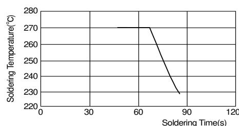
[Allowable Reflow Soldering Temperature and Time]
