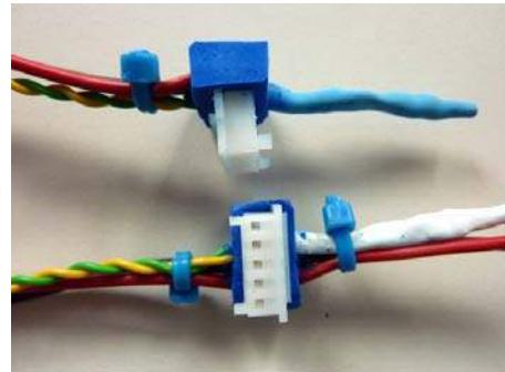
Sugru is the exciting new self-setting rubber that can be formed by hand. It moulds like play-dough, bonds to almost anything and turns into a strong, flexible silicone rubber overnight.
