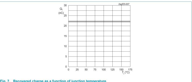
Fig. 7. Recovered charge as a function of junction temperature
