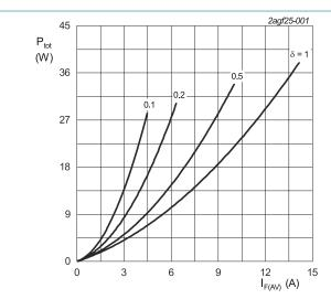
$I_{F(AV)} = I_{F(RMS)} \times \sqrt{\delta}$  $V_o = 0.997 \text{ V}; R_s = 0.1192 \Omega$
