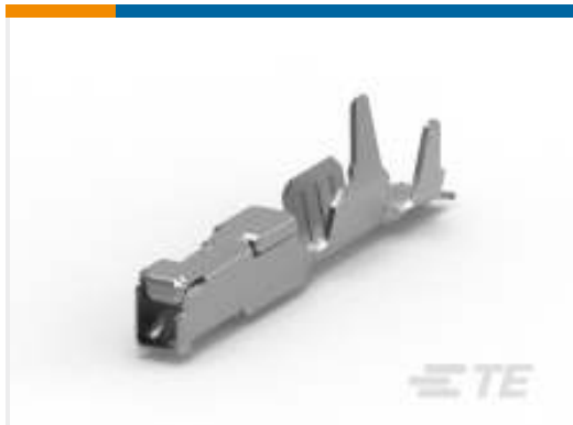
TE Part #2098762-2 Contact, female 0.64, 18AWG, CuN
