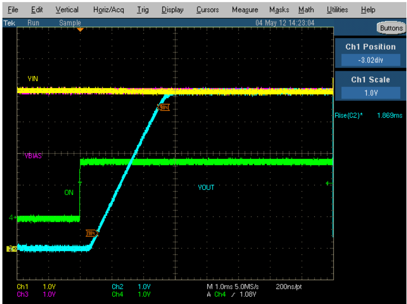
Figure 7. TPS22965EVM-023 Trise VIN = 5 V, ct = 1nF, and Load = 10 Ω
