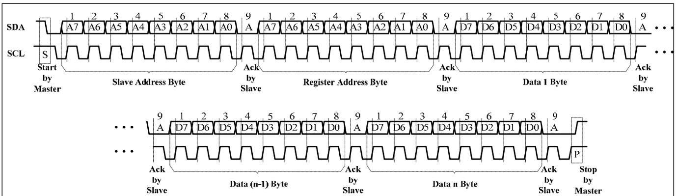
Figure 6 Writing to IS31FL3741 (Automatic address increment)
