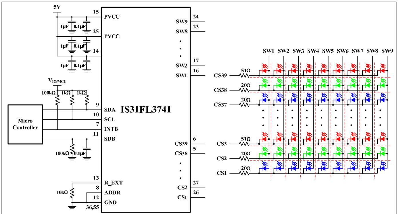
Figure 2 Typical Application Circuit (RGB Color: 13x9)
