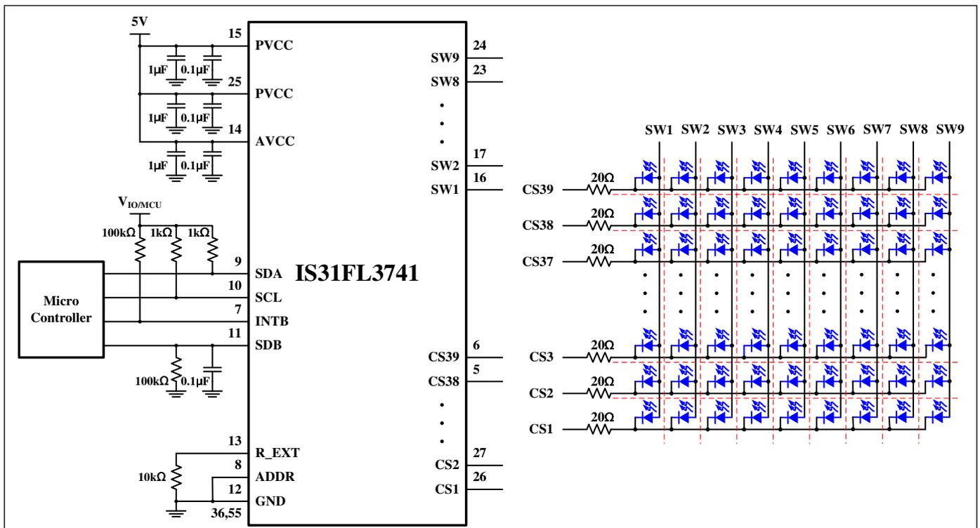
Figure 1 Typical Application Circuit (Single Color: 39×9)
