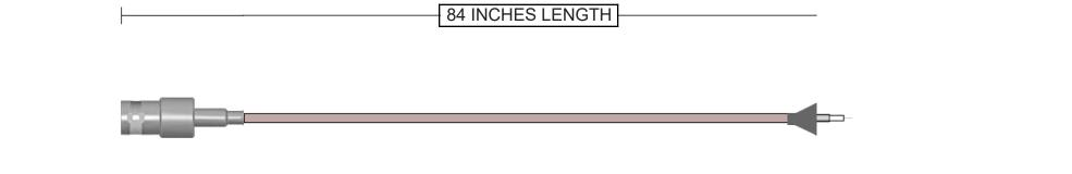
Connector A 112160 BNC Jack Straight Brass Nickel 50 Ohm RG-316 Continuity/Hi-Pot Connector B FA1-NZSJ-C01-0 FAKRA Jack Straight Brass Nickel + Heatshrink
