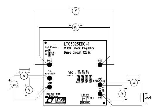
Figure 2. Proper Measurement Equipment Setup
