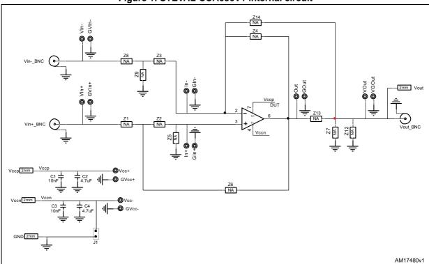
Figure 1. STEVAL-CCA036V1 internal circuit
