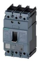
circuit breaker 3VA5 UL frame 125 breaking capacity class H 65kA @ 480 V 3-pole, line protection TM230, FTAM, In=15A overload protection Ir=15A fixed short-circuit protection Ii=10...20 x In nut keeper kit on both sides
