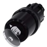
key-operated switch Siemens, 22 mm, round, plastic, lock number SSG10, with 2 keys, 2 switch positions O-I, latching, actuating angle 90°, 10:30h/13:30h, key removal O+I
