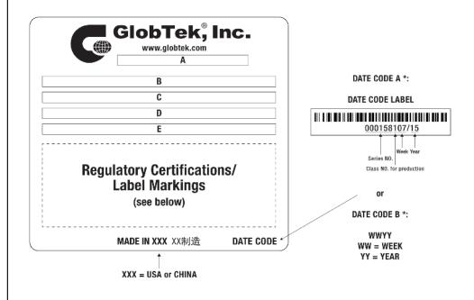
A=ICT/ITE Power Supply B=P/N: (料号) WR9MA2000MICB-F(R6W) C=Model (型号) GT-86120-1005-W2E D=Input (输入)100-240V-, 50/60Hz, 0.5A E=Output (输出)5.0 V == 2.0 A, 10.00W
