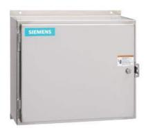
Mechanically held lighting contactor, Contactor amp rating 60Amp 0NC  $\_$  8NO poles, 208VAC 60HZ coil, Non-combination type, Enclosure NEMA type 12, Dust/drip proof for indoors
