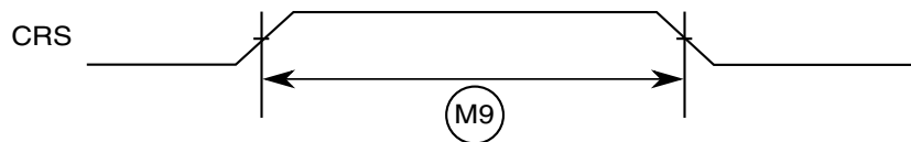
Figure 43. MII async inputs timing diagram
