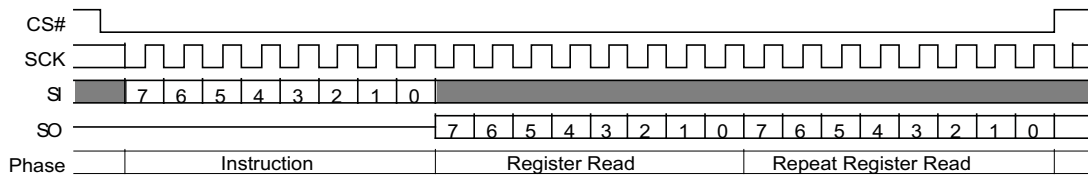
Figure 54. Read Bank Register (BRRD 16h) Command
