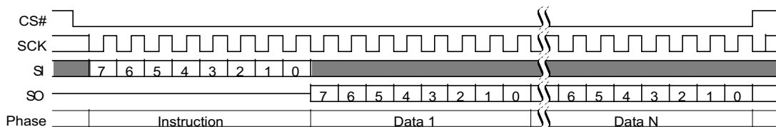
Figure 117. Password Read (PASSRD E7h) Command Sequence
