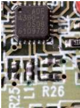
Figure 3. External Inductors and Resistors for ADF4360-7 Tank Circuit
