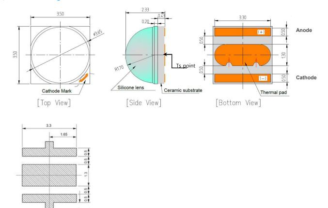
Measurement unit: mm Tolerance: ±0.13 mm
