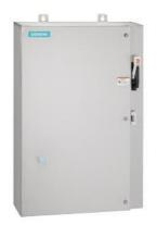
Non-reversing motor starter Size 2 1/2 Three phase full voltage Solid-state overload relay OLRelay amp range 25-100A 24VAC 50-60HZ coil Combination type 100A non-fusible disconnect Encl NEMA type 4X 316 S-steel Water/dust tight non-corrosive Extra-wide enclosure
