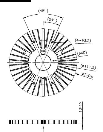
Assembly direction of customer's LED Module
