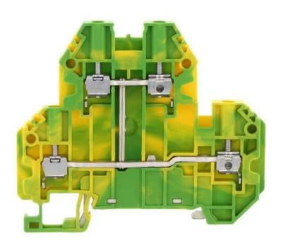
Protective-earth double-level terminal, Screw connection, Mounting type: Mounting rail TS 35/7.5, Rated cross-section: 2.5 mm², Width: 5.1 mm, Colour: Green-yellow
