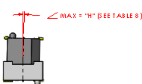
FINAL X AXIS ANGULAR MISALIGNMENT
