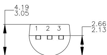
**Mechanical Dimensions (Continued)****Package****Dimensions in millimeters****TO-92 Formed Lead For T&R and Ammo Packing**
