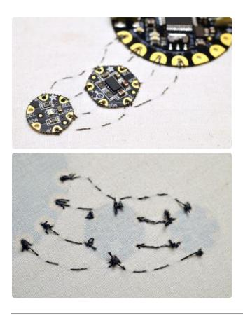
Stitching the sensor into a project is easyjust line up the sensor so its adjacent to the SDA/SCL pins on Flora or another I2C sensor, and stitch the four connections with conductive thread. This is covered in more detail in the Flora Accelerometer () guide and our Conductive Thread () guide.
