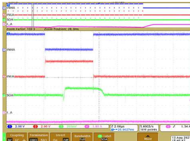
Figure 9-6. Driver PWM operation with feedback
