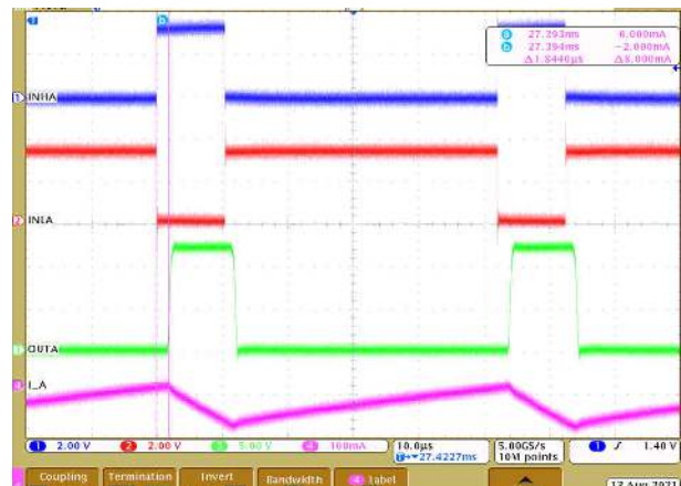
Figure 9-9. Driver delay compensation (1.8 μs)
