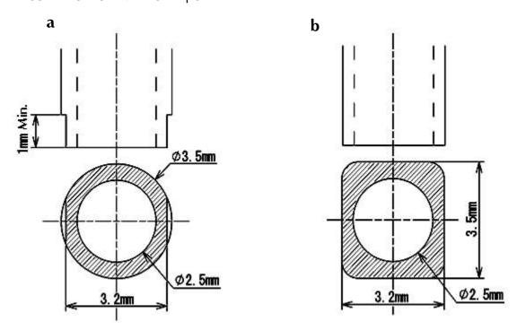
Nozzle with chamfering is recommended
