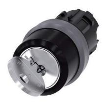
RONIS key-operated switch, 22 mm, round, plastic with metal front ring, lock number 455, with 2 keys, 2 switch positions O<I, momentary contact type, Actuating angle 45°, 10:30h/12h, key removal O, with laser labeling, upper case
