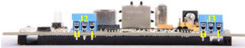
Figure 2-3. J2, J3 CAN Bus Interface (Screw Terminal)
