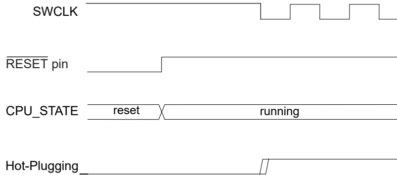
Figure 13-3. Hot-Plugging Detection Timing Diagram
