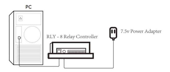
**NOTE**: If you directly connect to the computer, you will need to set a static IP. Going by RLY factory settings, you can set your computer IP to 192.168.1.x(x is 0~254 except 10), Subnetmask 255.255.255.0, gateway 192.168.1.1
