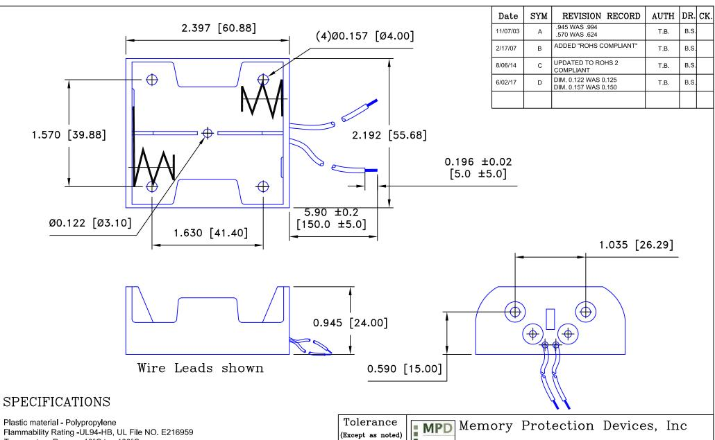
Flammability Rating -UL94-HB, UL File NO. E216959 Temperature Range: -10°C to +100°C Springs - Nickel Plated Spring Steel Wire - 26 AWG, UL1007, CSA, TR64, 300V, 80°C Rivets - Brass, Nickel Plated
