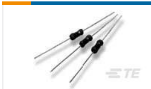
TE Part #3-1625885-2 1W SM M/OX 5% 1K2
