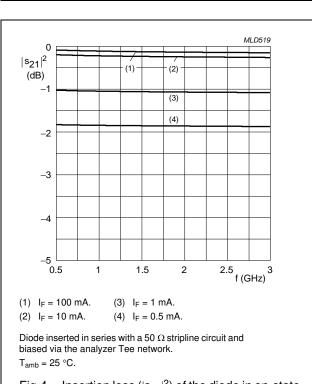
Fig.4 Insertion loss  $(|s_{21}|^2)$  of the diode in on-state as a function of frequency; typical values.
