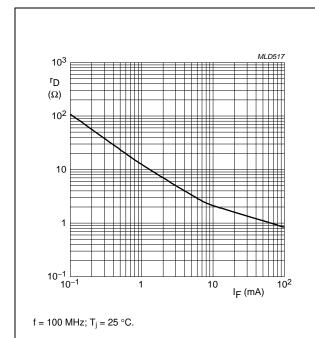
Fig.2 Forward resistance as a function of forward current; typical values.
