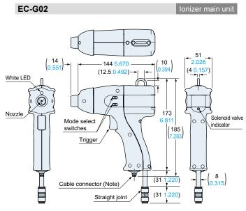
Note: An exclusive intermediate cable (oil-resistant, heat-resistant, bendingresistant type, Ø3.7 mm Ø0.146 in, 2 m 6.562 ft long) is attached.
