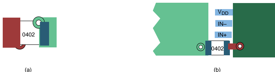
Figure 22. Typical Decoupling Capacitor Layouts
