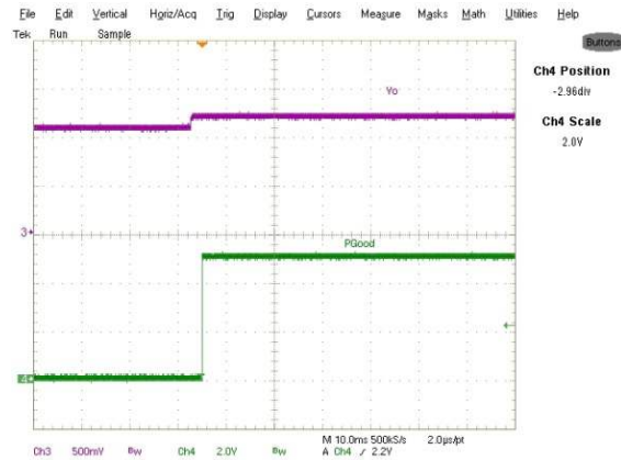
Figure 33 Start up with 1.06V Pre Bias, 0A Load Ch3: Vo, Ch4: P_Good
