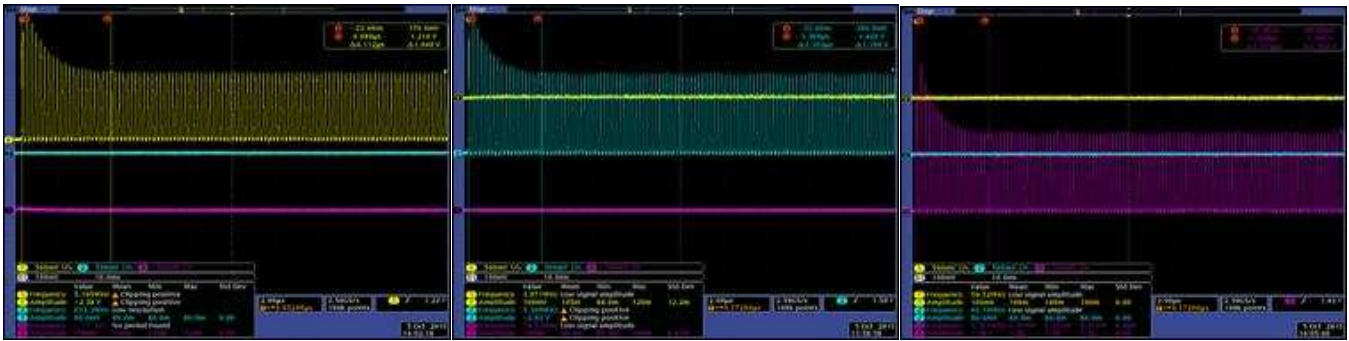
Figure 8. Proximity Startup Waveform (Yellow), Cap Touch Button 1/2 Startup Waveforms (Green, Magenta)
