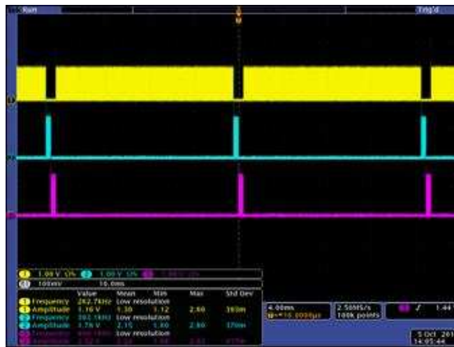
Figure 9. Sensor Multiplexing – Proximity (Yellow), Cap Touch Button 1 and 2 (Green, Magenta)
