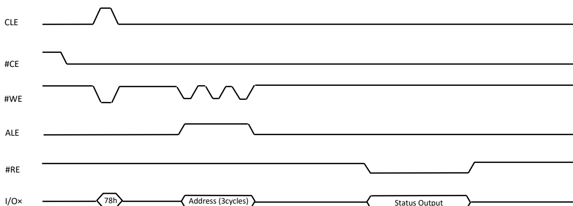
Figure 9-8 Read Status Enhanced (78h) Operation
