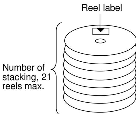
\* Insert cushion material in the empty spaces to secure reels.
