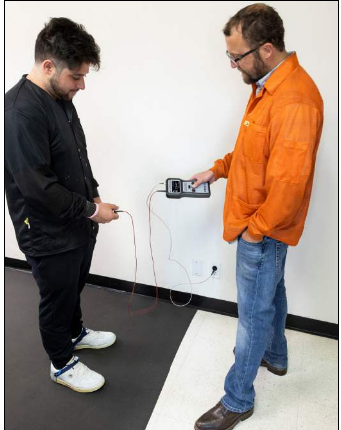
Figure 10. Using the Desco 19295 Handheld Electrode to measure Floor Materials and Footwear - Resistance Measurement in Combination with a Person (ANSI/ESD STM97.1)
