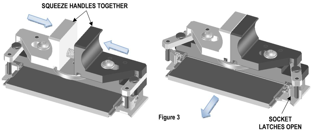
4. Release the extraction tool handles and remove the tool from the memory card socket.
