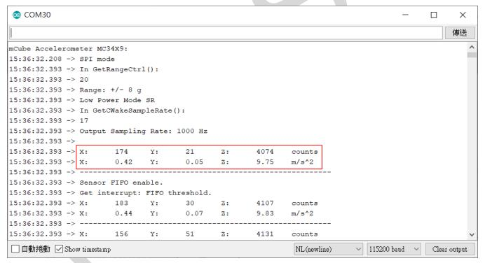
You will see the output from the serial terminal showing the current range scale and resolution of the sensor in the first three lines followed by two lines of output sensor data at some output data rate which depict "raw count" data for line 1: X: 174 Y: 21 Z: 4074 with 8G range, 16bit ADC resolution. Line 2 indicates the SI units for measuring acceleration as X: 0.42 m/s^2 Y: 0.05 m/s^2 Z: 9.75 m/s^2.
