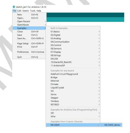
If you need the sensor running on SPI, please configure the bus as SPI in the MC34X9\_demo.ino shown as below. Otherwise, the default is I2C bus.
