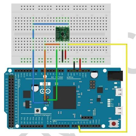
The EV3419A evaluation board can be easily wired to any microcontroller. This example shows a typical Arduino DUE platform. Please refer to the illustration below for connecting the related pins and then port the code to get the raw X, Y, Z sensor data.
