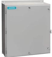
Non-reversing motor starter, Size 3 1/2, Three phase full voltage, Solid-state overload relay, OLRelay amp range 50-200A, 550/575 600 50/60HZ coil, Non-combination type, Enclosure type 12, Dust/drip proof for indoors, Extra-wide enclosure
